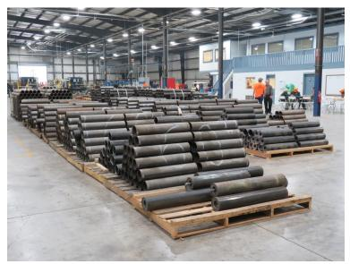
Steel Tubes Ready to Have End Caps Fitted and Welded
