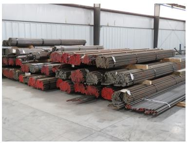
Steel Rods for Roll Shafts
