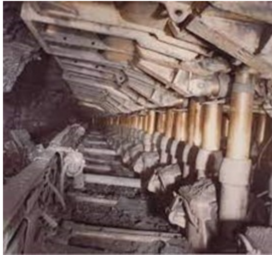
Figure 7 - Dowty Roofmasters Supporting the Roof in a 48" Thin Coal Seam
